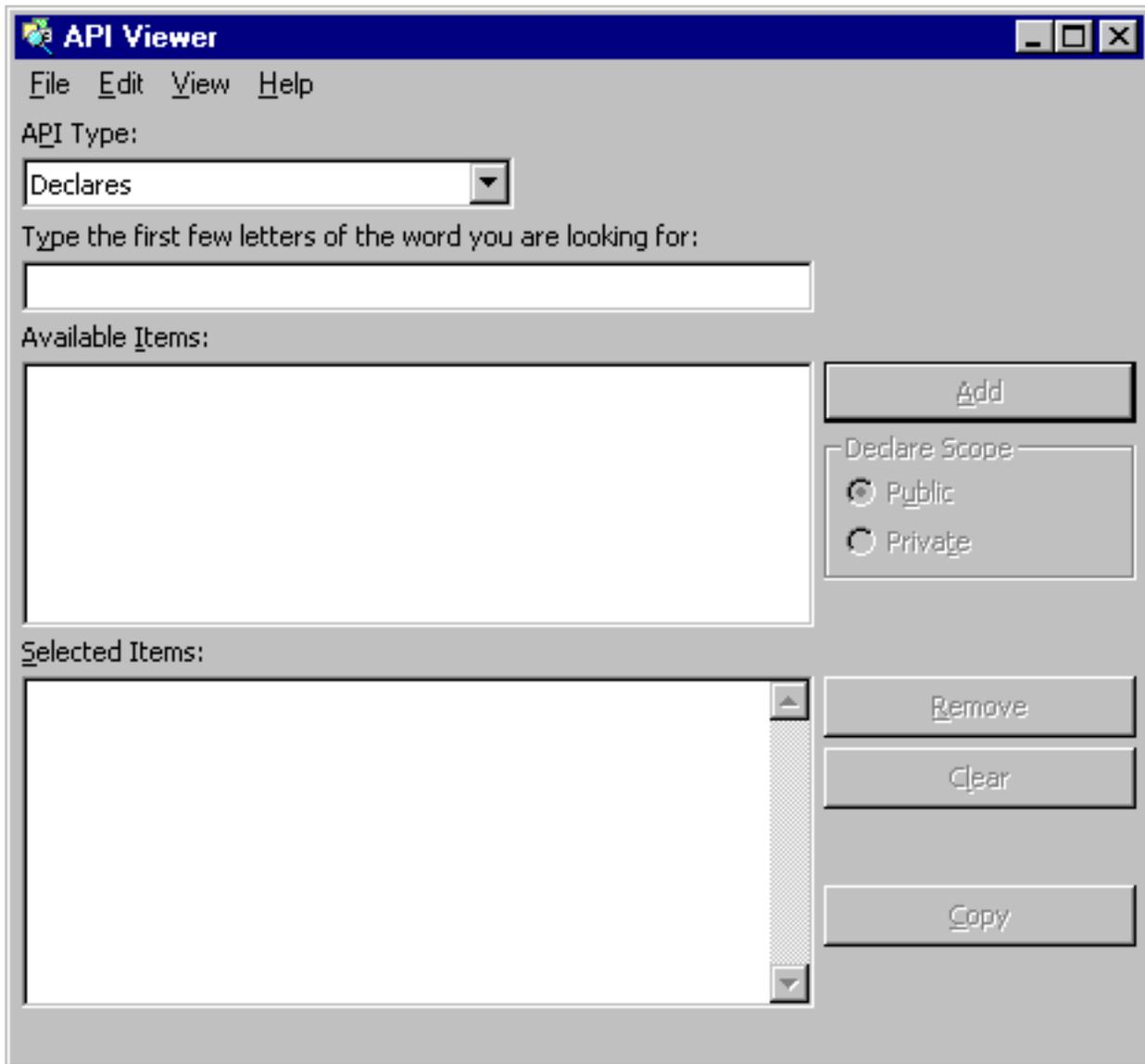
which at first glance can be a little imposing. The API Text Viewer is just an application that allows you to view the contents of one of three text files installed with VB, that provide the barest form of documentation on the functions and procedures contained in the DLL's supplied with Windows. Before we can do anything with the API Text Viewer, we need to make a selection of one of the text files. We can do that by selecting File-Load Text File from the API Text Viewer menu bar...
