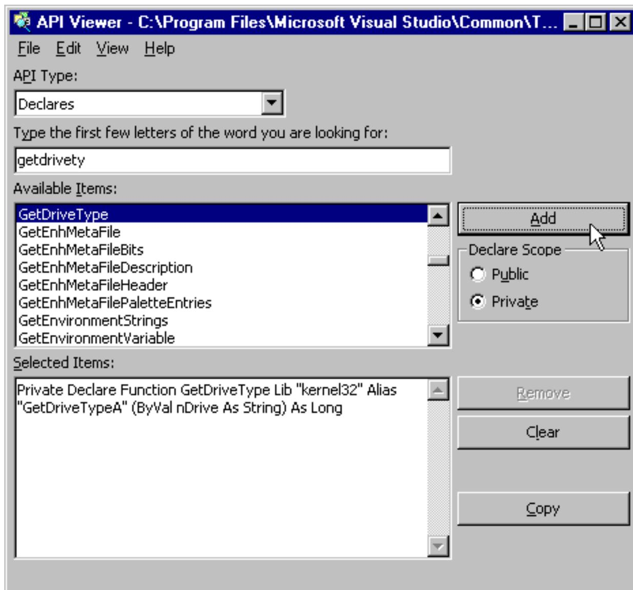
At this point, I'll create a new Visual Basic project with a single form containing a textbox and a command button, and copy and paste the Declare statement into the General Declarations Section of the form.
